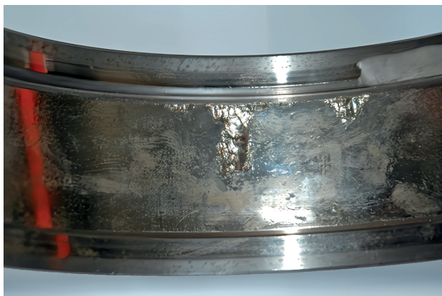
Figure 3: The description of White Etching Cracking is near-identical to hydrogen wear phenomenon
