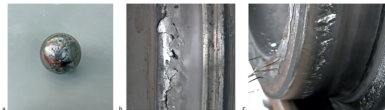
Figure 2: Examples of hydrogen wear on various surfaces. a. Hydrogen wear on an SKF bearing ball, b. and c. A railway wheelset that's been worn down by the absorption of hydrogen during the braking process
