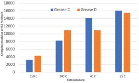
Figure 2: Complex modulus at 0.1% Strain for the lithium complex greases at various temperatures.
