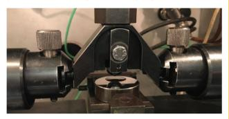
Picture 1: Shows the oil sample between the Disc and Ball in SRV-rig.
