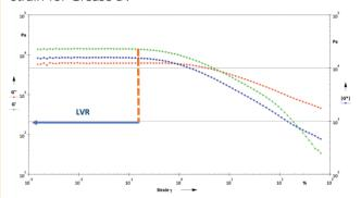
Figure 1: Elastic modulus, viscous modulus and complex modulus as functions of strain.
