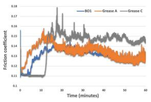
Figure 4: Measured friction coefficient as a function of time for BO1, Grease A and Grease C.
