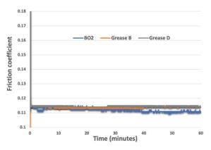
Figure 5: Measured friction coefficient as a function of time for BO2, Grease B and Grease D.
