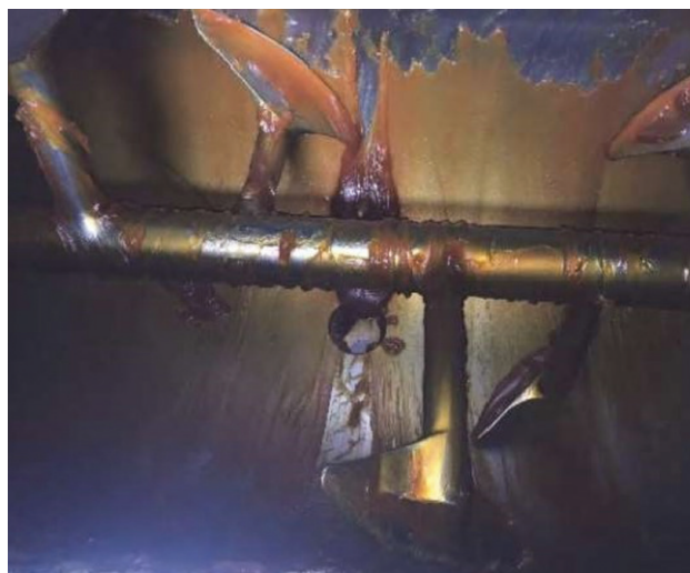
Figure 3: Inside view of the new modified reactor with mixing arms
