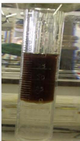
Figure 6. Strong water separation for fresh and thermally aged oils
