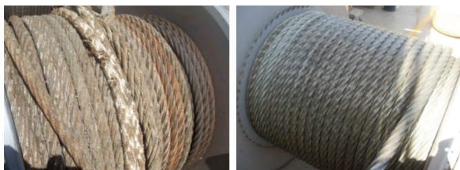
Figure 2. Without proper lubrication wire ropes degrade and lose longevity
