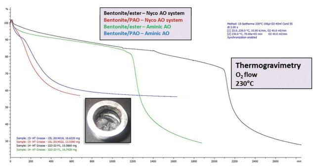
Figure 7. PAO 40 and ester based greases, thermogravimetric analysis, 230°C
