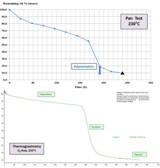
Figure 4. Pan test at 230°C and thermogravimety of NYCOBASE 9600X with NYCOPERF A0337
