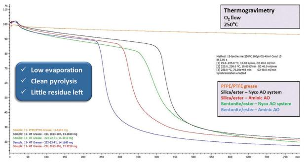
Figure 5. Thermogravimetric analysis, 250°C
