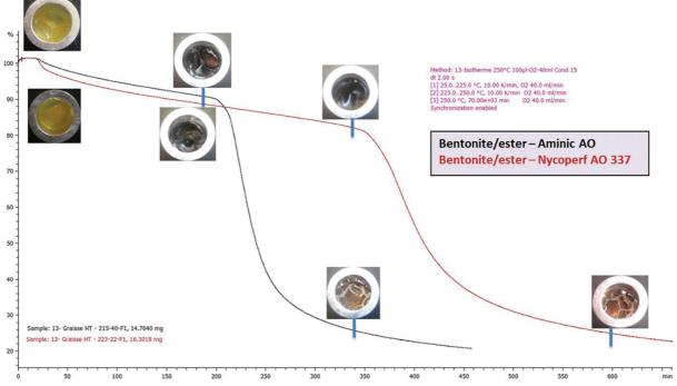
Figure 6. Ester based grease aspect before and after Induction Time, 250°C
