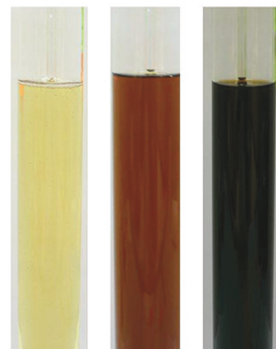
Figure 2. Visual assessment of the deposit control characteristics of two compressor oils that have been aged in a modified ASTM D2893B test.
